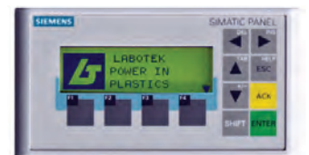
Siemens S7 series control DFD 100-8500
