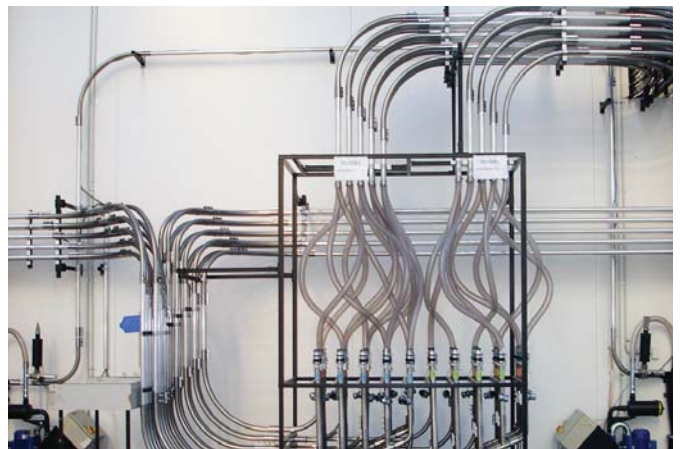
Example, Coupling station, 20 inlets/60 outlets
