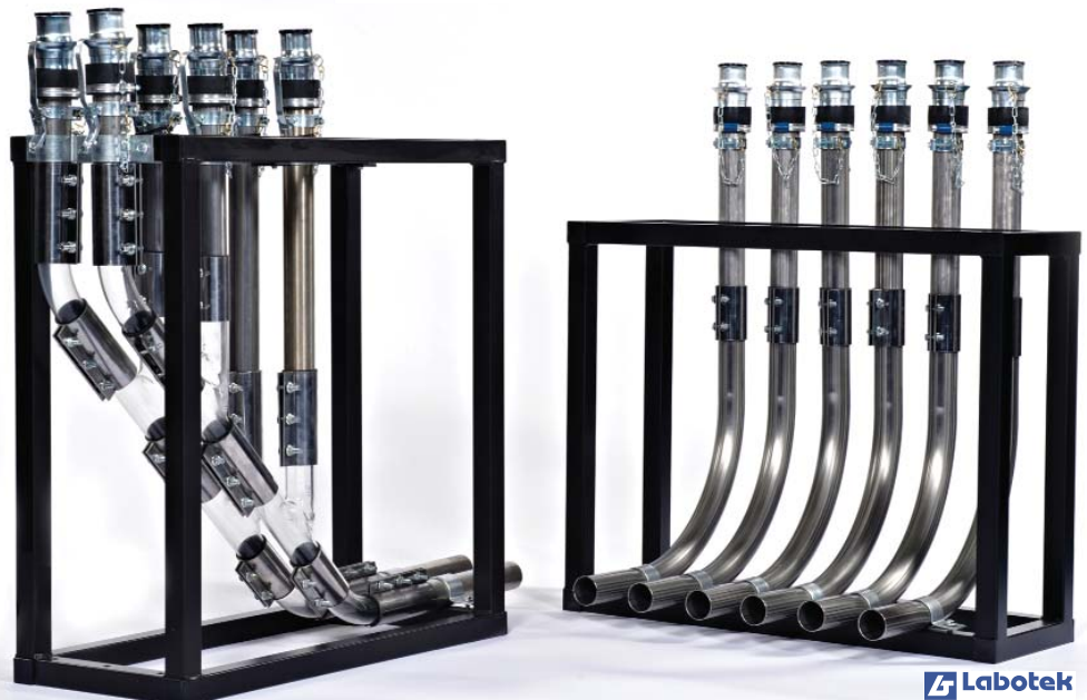
Example, Coupling station, 20 inlets/60 outlets
