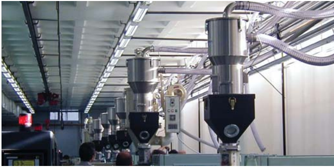
Vacuum receivers type SVR and insulated hoppers
